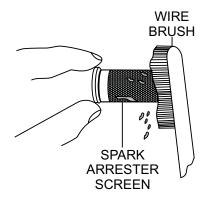
Figure 31. Cleaning The Spark Arrester
